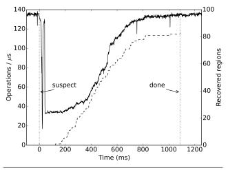
**Figure 14.** TATP throughput when optimizing for rereplication delay
