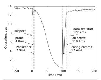
Figure 11. TATP performance timeline with CM failure
