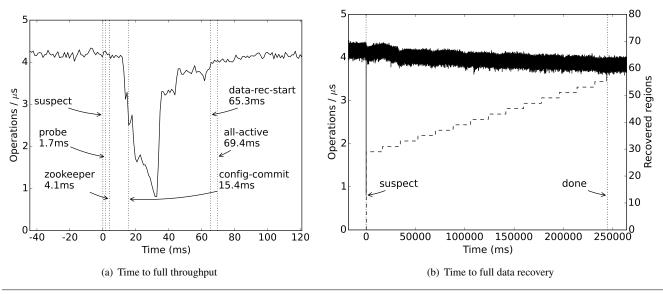
Figure 10. TPC-C performance timeline with failure
