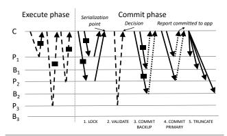
**Figure 4.** FaRM commit protocol with a coordinator C, primaries on  $P_1$ ,  $P_2$ ,  $P_3$ , and backups on  $B_1$ ,  $B_2$ ,  $B_3$ .  $P_1$  and  $P_2$  are read and written.  $P_3$  is only read. We use dashed lines for RDMA reads, solid ones for RDMA writes, dotted ones for hardware acks, and rectangles for object data.
