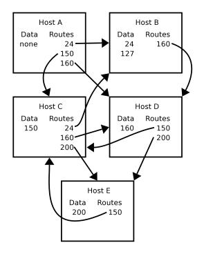
For example, host B's routing table contains an entry with key 160 referring to host D, and B's data store contains two files, one with key 24 and one with key 127.
