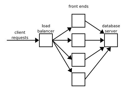
The load balancer sends HTTP requests to the front ends in round-robin order. The front ends communicate with the database server using UDP RPCs. Each client HTTP request involves the front end sending just one RPC to the database server. The front ends do not re-send these RPCs; if the front end gets no response after 100 seconds, it sends an error message to the HTTP client.
